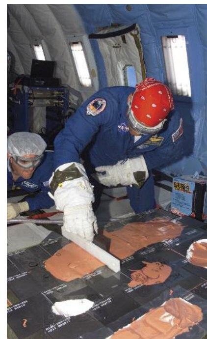
Astronauts Robert Curbeam (foreground) and Rex Walheim (background) simulate tile repair, using materials and tools developed after the Space Shuttle Columbia accident, on board the zero-gravity training aircraft KC-135.
