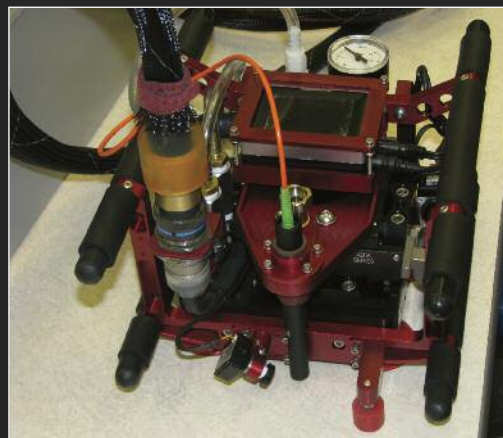
The Portable Handheld Optical Window Inspection Device is vacuum attached to a window such that the small camera and optical sensor (black tube) were aimed at a defect.
