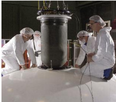
Technicians shown installing igniter used to initiate the propellant burn in a forward motor segment. The igniter was a small rocket motor loaded with propellant that propagated flame down the bore of the motor.
