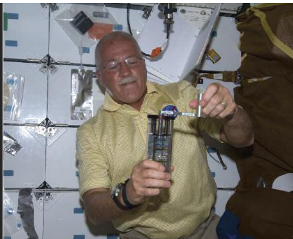
Astronaut John Phillips activating a Fluid Processing Apparatus containing tubes of microorganisms on STS-119 (2009).
