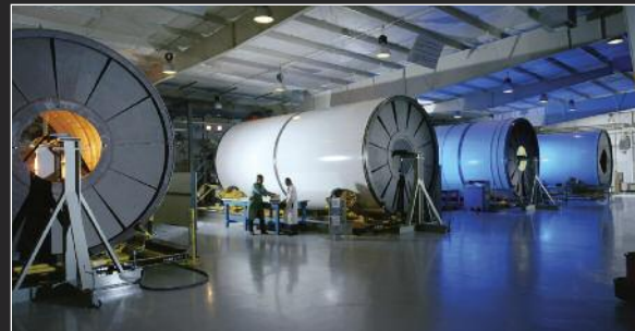
Technicians process the solid rocket motor case segments at the ATK case lining facility in Utah.
