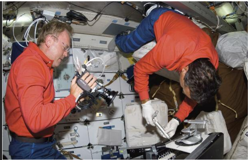
Astronaut Andrew Thomas (left) watches as Charles Camarda tests the reinforced carbon-carbon plug repair (STS-114 [2005]).
