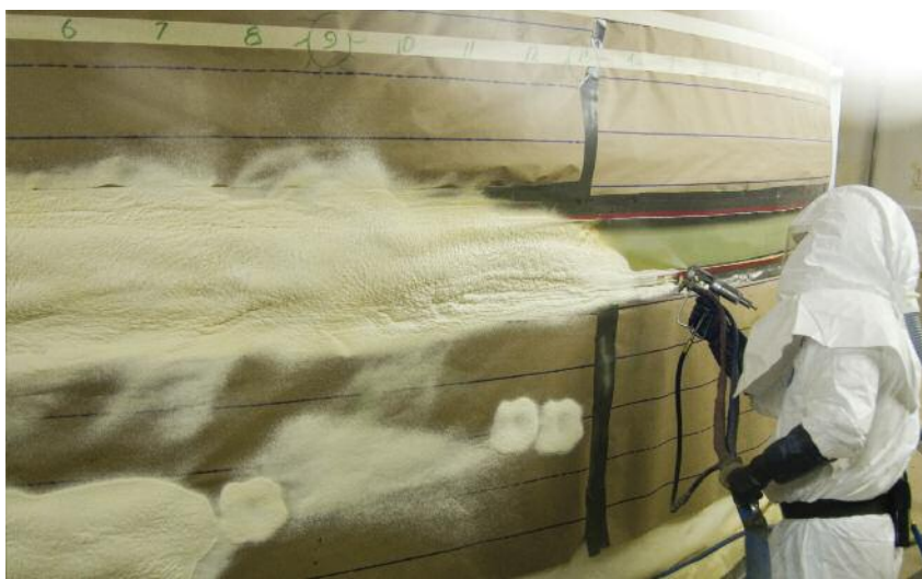
A technician at NASA's Michoud Assembly Facility sprays the flange that connects the intertank and liquid hydrogen tank. Stepanfoam® BX-265 was sprayed manually on closeout areas, exterior tank feedlines, internal tank domes, closeout areas of mating External Tank subcomponent surfaces, and small subcomponents.
