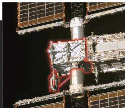
Discovery (STS-116) delivered P5 truss.
