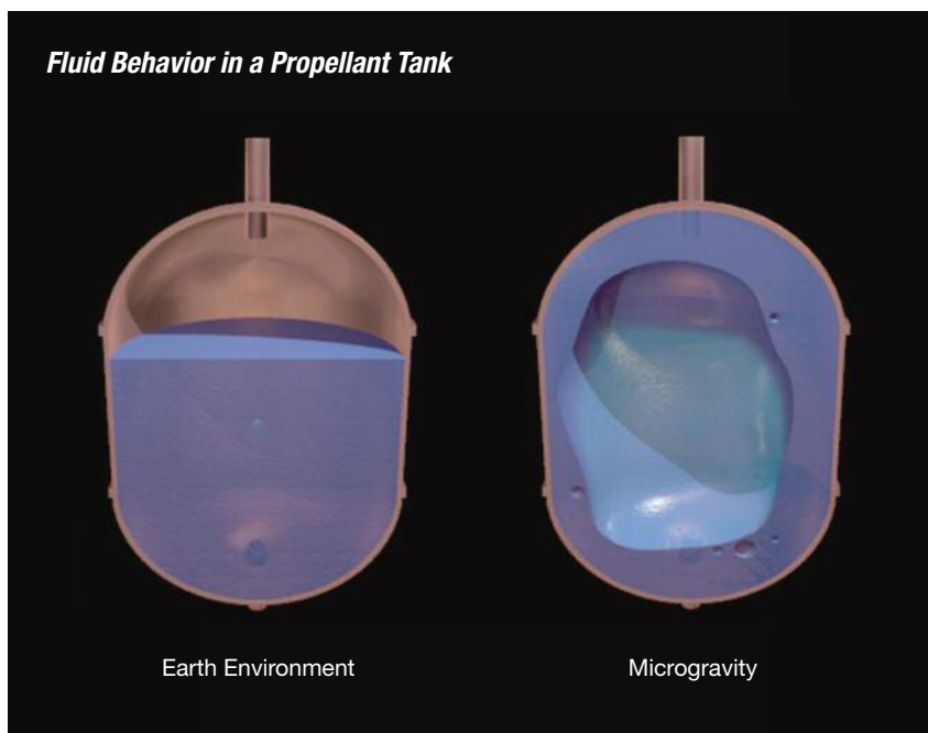
One of the earliest concerns about fluid behavior in microgravity was the management of propellants in spacecraft tanks as they orbited the Earth. On the ground, gravity pulls a fluid to a bottom of a tank (Earth environment, left). In orbit, fluid behavior depends on surface tension, viscosity, wetting effects with the container wall, and other factors. In some cases, a propellant can wet a tank and leave large gas bubbles in the center (microgravity, right). Similar problems can affect much smaller experiments using fluids in small spaces.
