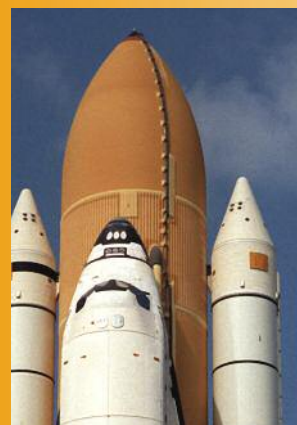
Insulating foam covers the External Tank.
