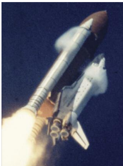
This photo shows clouds enveloping portions of the vehicle (STS-34 [1987]) during ascent. When the launch vehicle was in the transonic regime, shocks formed at various positions along the vehicle to recompress the flow, which greatly impacted the structural loads and aerodynamics. Such shocks, which abruptly transition the flow from supersonic to subsonic flow, were positioned at the trailing edge of the condensation “clouds” that could be seen enveloping portions of the vehicle during ascent. These clouds were created in localized areas of the flow where the pressure and temperature conditions caused the ambient moisture to condense.
