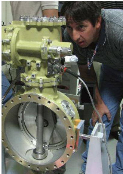
At the Shuttle Logistics Depot, Rick Zeitler assesses the cycling of a main propulsion fill and drain valve after a valve anomaly during launch countdown caused a scrub.
