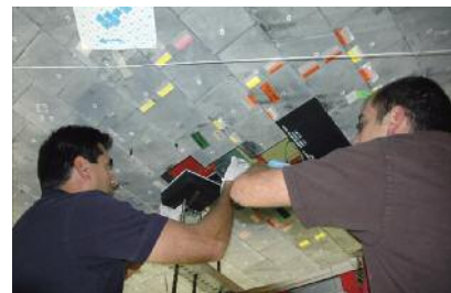
Prior to the launch of STS-119 (2009), Discovery gets boundary layer transition tile, which monitors the heating effects of early re-entry at high Mach numbers.
