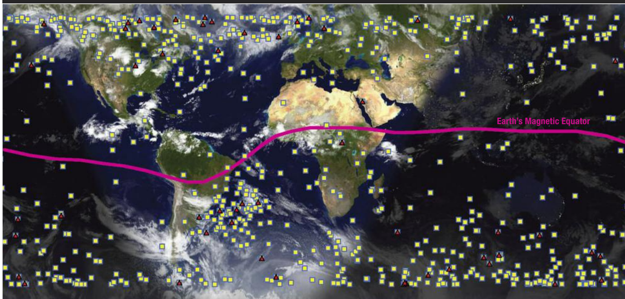
Single event upsets are indicated by yellow squares. Multi-bit single event upsets are indicated by red triangles. In these single events, anywhere from two to eight bits were typically upset by a single charged particle.
