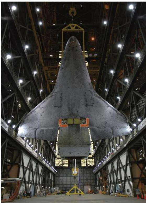
This view of the suspended Orbiter Discovery shows the underside covered with Thermal Protection System tiles.
