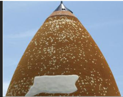
ET-124 damage repairs, post storm.
