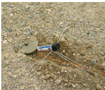
The Thiokol de-mining flare used excess shuttle propellant resulting from Solid Rocket Motor casting operations to burn through land mine casings and safely ignite the explosives contained within. The flares were activated with an electric match or a pyrotechnic fuse.
