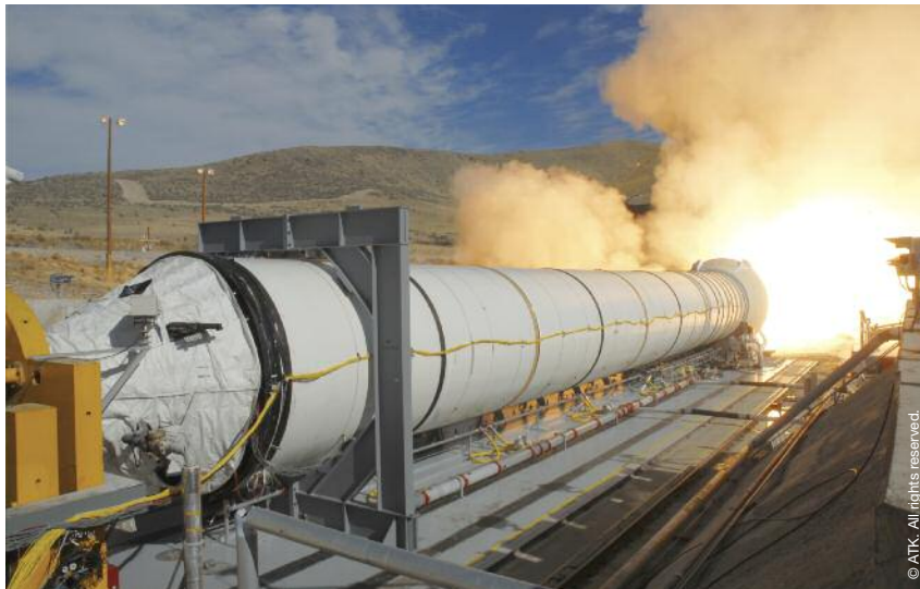
The two shuttle reusable solid rocket motors, which stood more than 38 m (126 ft) tall, harnessed 29.4 meganewtons (6.6 million pounds) of thrust. The twin solid-fueled rockets provided 80% of the thrust needed to achieve liftoff.
