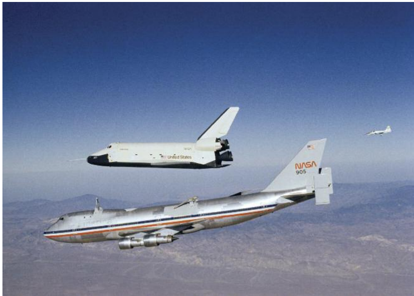
The Space Shuttle Enterprise was used to conduct approach and landing testing (1977) at the Dryden Flight Research Center, California. In the five free flights, the astronaut crew separated the spacecraft from the Shuttle Carrier Aircraft and maneuvered to a landing. These flights verified the Orbiter's pilot-guided approach and landing capability and verified the Orbiter's subsonic airworthiness in preparation for the first crewed orbital flight.
