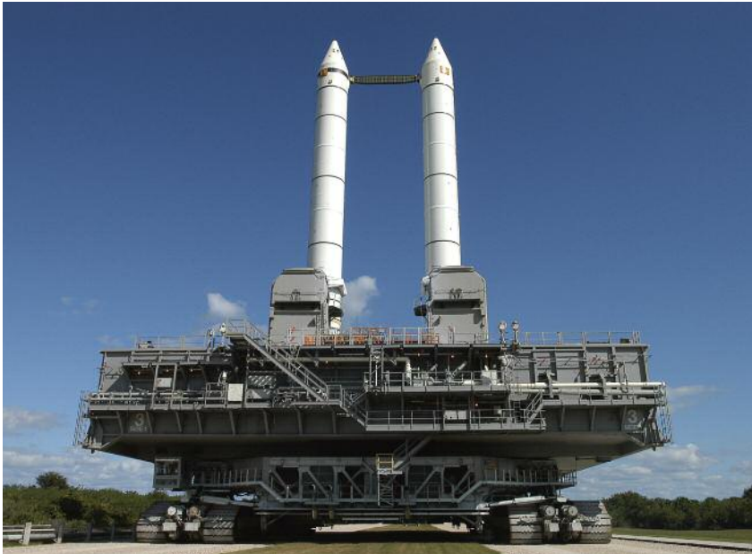
Rollout tests of the Solid Rocket Boosters. Mobile Launcher Platform number 3, with twin Solid Rocket Boosters bolted to it, inches along the crawlerway at various speeds up to 1.6 km (1 mile) per hour in an effort to gather vibration data. The boosters are braced at the top for stability. Data from these tests, completed September 2004, helped develop maintenance requirements on the transport equipment and the flight hardware.
