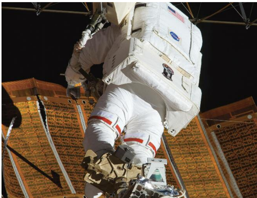
Contingency extravehicular activity: Astronaut Scott Parazynski, atop the Space Station Robotic Arm and the Shuttle Robotic Arm extension, the Orbiter Boom Sensor System, approaches the International Space Station solar arrays to repair torn sections during STS-120 (2009).
