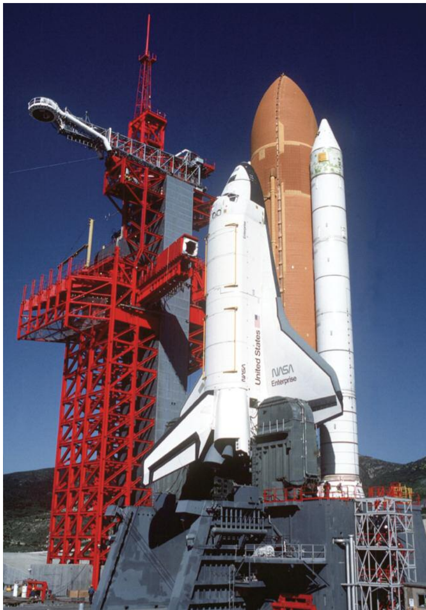
Space Shuttle Enterprise on Space Launch Complex 6 during pad checkout tests at Vandenberg Air Force Base in 1985. Enterprise was the Orbiter built for the Approach and Landing Tests to prove flightworthiness. It never became part of the shuttle fleet.
