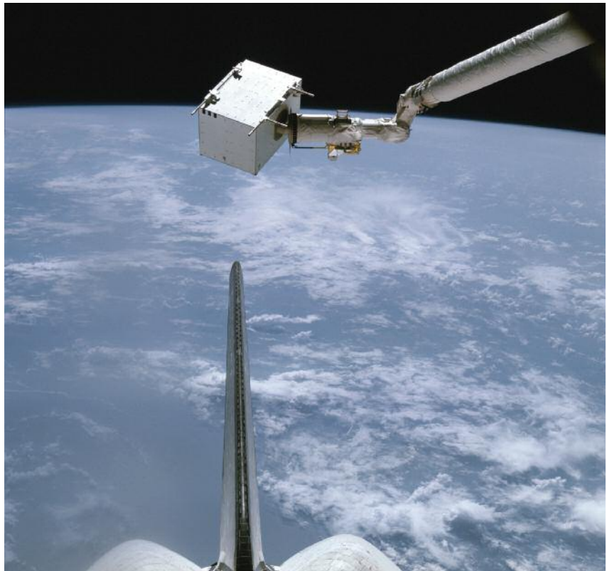
The Atlantic Ocean southeast of the Bahamas is in the background as Columbia's Shuttle Robotic Arm and end effector grasp a multi-instrument monitor for detecting contaminants. The experiment, called the Induced Environment Contaminant Monitor, was flown on STS-4 (1982). The tail of the Orbiter can be seen below.
