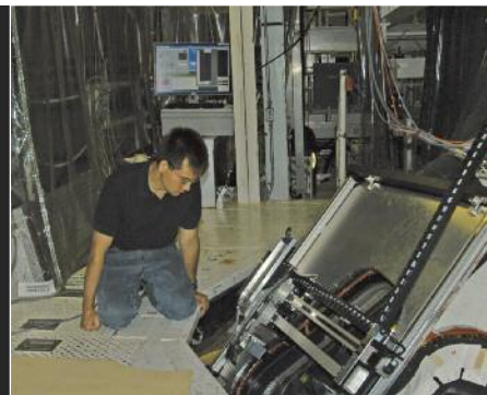
Bradley Burns, lead engineer in the development of the window inspection tool, monitors its progress as it scans an Orbiter window.
