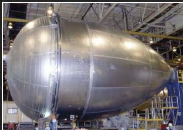
Liquid oxygen tank.
