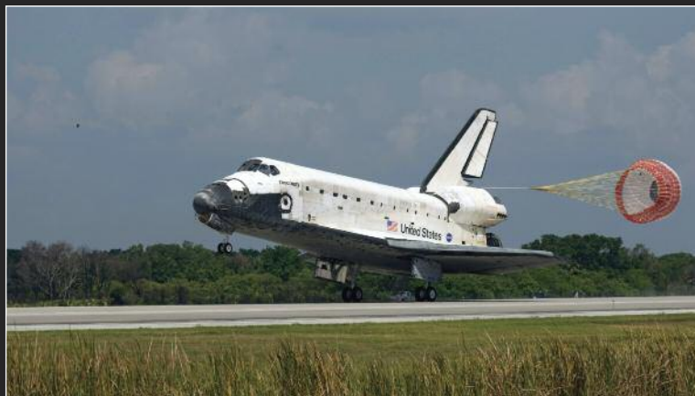
Space Shuttle Discovery's drag chute is deployed as the spacecraft rolls toward a stop on runway 15 of the Shuttle Landing Facility at Kennedy Space Center, concluding the 14-day STS-124 mission to the International Space Station.
