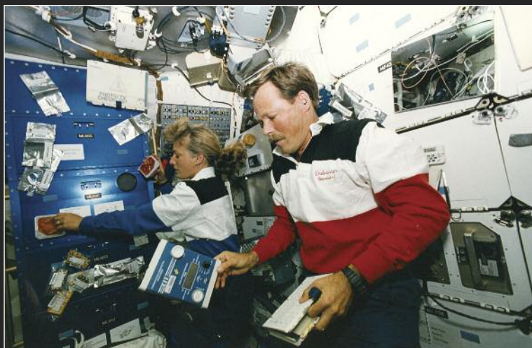
Commander Robert Gibson and Astronaut Jan Davis check the combustion product analyzer during STS-47 (1992).
