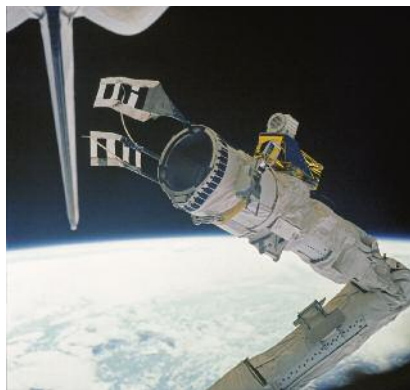
Fly swatting—On STS-51D (1985), the spacecraft sequencer on the Leasat-3 satellite failed to initiate antenna deployment, spin-up, and ignition of the perigee kick motor. The mission was extended 2 days to make the proper adjustments. Astronauts David Griggs and Jeffrey Hoffman performed a spacewalk to attach “fly swatter” devices to the robotic arm. Rhea Seddon engaged the satellite's lever using the arm and the attached “fly swatter” devices.
