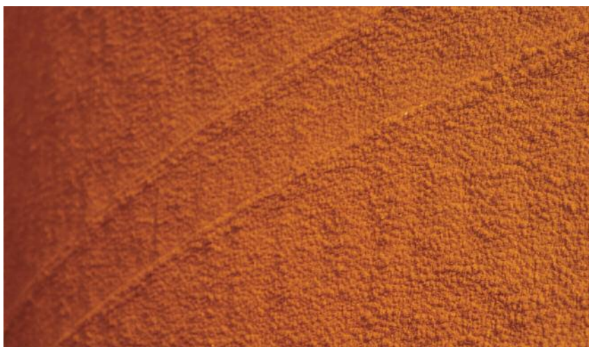
The key to the External Tank's foam Thermal Protection System insulating properties was its cellular structure, creating millions of tiny bubble-like foam cells. The sprayed foam (NCFI 24-124) can be seen here after application to an area of the tank's aluminum "acreage," consisting of the liquid oxygen tank, liquid hydrogen tank, and intertank.
