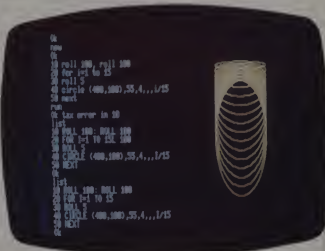
It is easy to debug graphics programs as the text screen and graphics screen are independent. Here, we have written a simple
