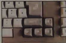
RETURN key is double size and cursor control keys are arranged reasonably logically.
