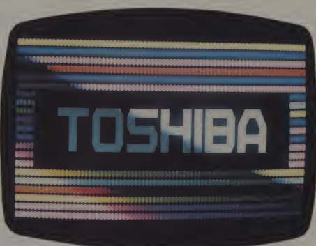
High resolution screen displays 600 x 240 pixels in eight colors.
